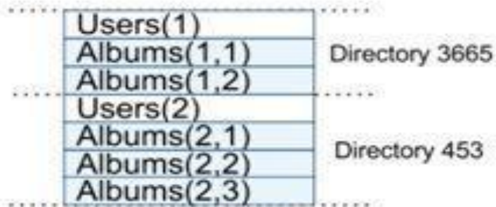
Figure 4: Example Spanner schema for photo metadata, and the interleaving implied by INTERLEAVE IN.
